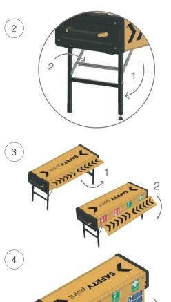
Lift the unit by the handles (1 person each end) and lower both sets of legs until fully unfolded (1). Push red Handle to lock in position (2).
